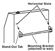
Figure 11 - Mounting Heater Onto Mounting Bracket
